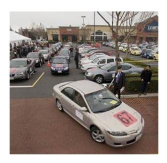
Cars at the Mobile Century command center in Union City head out on their 10-mile driving route on I-880. The drivers, all UC Berkeley students, carried GPS-enabled cell phones that transmitted speed and position information to researchers at the command center, creating a nearly real-time picture of traffic flow. (Paul Kirchner Studios photo)
