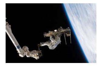
ESA astronaut Christer Fuglesang during the second spacewalk of the STS-116 mission to the International Space Station. Fuglesang stands on a platform at the end of the Station's robotic arm, Canadarm2, during operations to relocate two CETA carts. Credits: NASA
