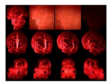
Top row: Erasing of the hologram; Mid and bottom rows: 3D images shown from different angles, demonstrating horizontal parallax. Credit: UA
