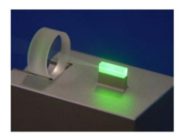
Squeezed light source: a crystal that is illuminated with green light places photons of an infrared laser beam (not visible) in a specific order, thereby reducing the photon noise in that infrared laser. Image: Roman Schnabel / MPI for Gravitational Physics
