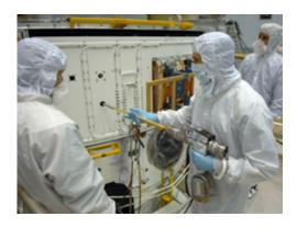
Servicing Mission 4 astronaut Drew Feustel trains with fellow astronauts and Hubble engineers in the clean room at NASA's Goddard Space Flight Center. Feustel is using a computer-controlled power tool, called the Pistol Grip Tool, to install the Wide Field Camera 3 into a high-fidelity Hubble model. Credit: NASA
