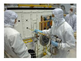
Servicing Mission 4 astronaut Drew Feustel trains with fellow astronauts and Hubble engineers in the clean room at NASA's Goddard Space Flight Center. Feustel is using a computer-controlled power tool, called the Pistol Grip Tool, to install the Wide Field Camera 3 into a high-fidelity Hubble model. Credit: NASA
