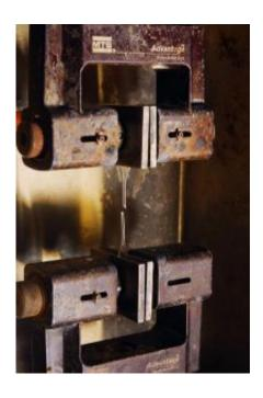
Inside a thermo-mechanical test frame, a shape-memory polymer fractures as it stretches past its deformation limit. This testing allows the researchers to determine the maximum possible shape change from the permanent to temporary shape and vice versa. Credit: Gary Meek
