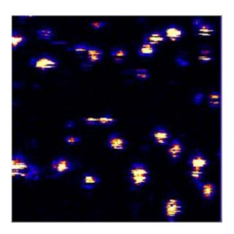
JILA scientists have found a way to suppress the blinking problem in quantum dots by bathing them in a chemical solution. This animated image, which demonstrates the basic blinking phenomenon, is made from a series of 40 images taken about one minute apart. Quantum dots actually blink on time scales ranging from millionths of a second to tens of seconds or longer. Credit: K Kuno/JILA
