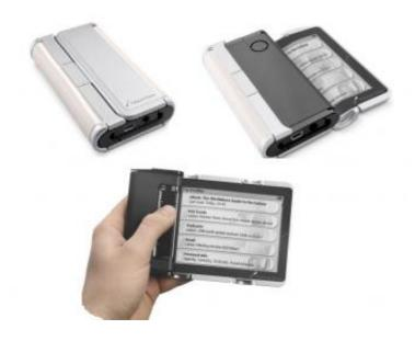
The Readius&acute e-paper display rolls out of a normal-sized cell phone. Image credit: Polymer Vision.
