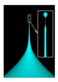
This image, created using a modeling technique called finite element computation, shows a droplet forming from a liquid that has been exposed to an electric field. Chemical engineers at Purdue are the first to mathematically describe precisely how the process forms droplets, an advance that could have applications in areas ranging from manufacturing to medical diagnostics. Credit: Purdue University, School of Chemical Engineering
