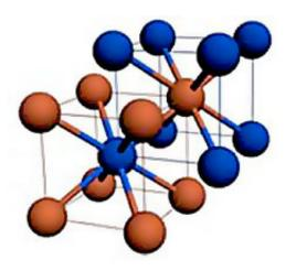
"Body-centered-cubic" unit cells of the 3-D nanoparticle crystals. One type of nanoparticle occupies each corner of the cube and a second type of nanoparticle is located centrally inside. These unit cells, measuring tens of nanometers, form a repeating lattice that extends more than a micron (1,000 nanometers) in three dimensions.
