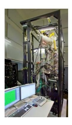
TEAM 0.5, the world's best transmission electron microscope, is being assembled at the National Center for Electron Microscopy. (Photo Roy Kaltschmidt, Berkeley Lab CSO)
