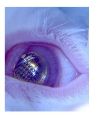
Contact lenses with metal connectors for electronic circuits were safely worn by rabbits in lab tests. Credit: University of Washington
