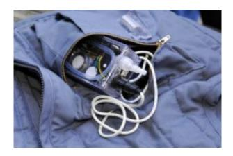
A sensor system, which fits in the pocket of a vest, continuously monitors the air around persons prone to asthma attacks. Researchers at the Georgia Tech Research Institute hope the system helps them better understand the causes of asthma attacks. Georgia Tech Photo: Gary Meek
