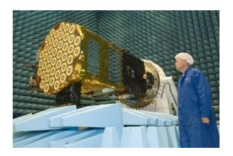
Galileo In-Orbit Verification (IOV) satellite under test at Thales Alenia Space, Toulouse. Credits: Thales Alenia Space
