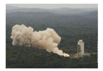
P80 static firing test being performed on 4 December 2007, using the solid booster test stand (Bâtiment d'Essai d'Accélérateur à Poudre - BEAP) at the Guiana Space Centre, Europe's Spaceport in Kourou, French Guiana. This is the same facility that is used for firing tests on Ariane 5's solid-propellant boosters. Credits: ESA / CNES / CSG-SOV
