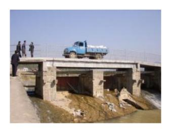
The 10 meter long modern bamboo bridge under 8 ton traffic loading testing. Credit: Yan Xiao
