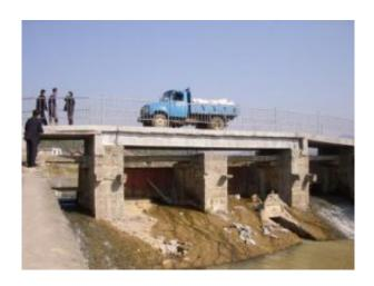
The 10 meter long modern bamboo bridge under 8 ton traffic loading testing. Credit: Yan Xiao
