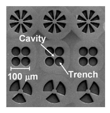
This electron micrograph image of the single-photon sources developed at UCSB shows the etched trenches that leave behind large, 20-micron cavities. The different geometries influence the shape of the confined light field inside the cavity and thus dictate the polarization of the emitted photons. Image credit: Stefan Strauf, et al.
