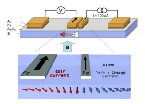
The illustration shows the lateral device with the non-local detection, which was used to demonstrate the electrical injection, detection and modulation of spin current in silicon. A charge current of spin-polarized electrons follows the applied voltage and flows to the right, while a pure spin current flows to the left. Credit: NRL
