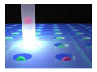
MIT has developed a new system for sorting cells that involves special "traps" in a silicone layer bonded to a microscope slide. Cells with specific properties are then levitated out of their traps using the pressure of a beam of targeted light from a low-cost laser. A flowing fluid then sweeps the selected cells off to a separate reservoir Image courtesy / Joseph Kovac, MIT
