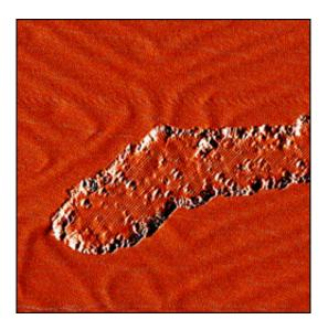
A scanning tunneling microscopy (STM) image taken of ceria nanoparticles on a gold surface. Size: 40 x 40 nanometers. Credit: Brookhaven National Laboratory
