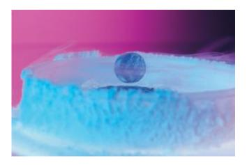
This photo shows a magnet levitating above a high-temperature superconductor, cooled with liquid nitrogen. A persistent electric current flows on the surface of the superconductor, effectively forming an electromagnet that repels the magnet. The expulsion of an electric field from a superconductor is known as the "Meissner Effect." Credit: Los Alamos National Laboratory
