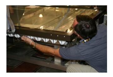
NIST technician Dana Strawbridge bolts the top frame of the map encasement to its base during a test sealing of the encasement prior to shipping to the Library of Congress. Credit: NIST
