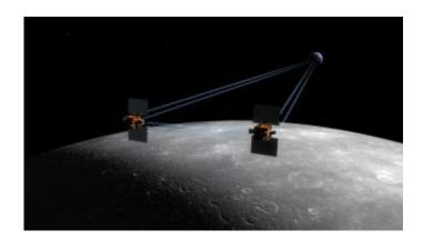
Artist concept of Grail mission. Grail will fly twin spacecraft in tandem orbits around the moon for several months to measure its gravity field in unprecedented detail. Image credit: NASA/JPL
