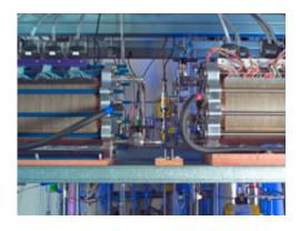
Regenerative fuel cell stacks at NASA Glenn. Credit: NASA
