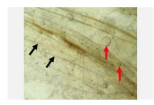
Photo of mica from an abandoned mica mine, with water between some layers, showing edges of mica sheets [e.g., black arrows] and air bubbles in the water [red arrows] and brown bands of organic crud and dirt. Credit: Helen Greenwood Hansma, UC Santa Barbara
