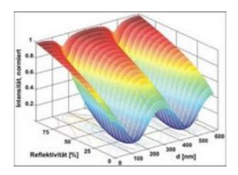
Intensities of the interferences of common Fizeau interferometers, in this example calculated for a reference surface with a reflectivity of 0.5 and test sample surfaces with varying reflectivity between 0 and 100% and a variation of the distance d between test sample and reference piece over a wavelength ( $\lambda$  = 633 nm). The new method avoids the strong dependence of the intensity profile and the contrast on the reflectivity of the test sample's surface. Credit: PTB
