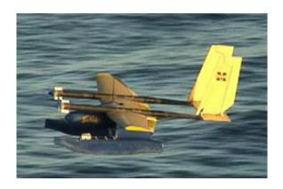
Flying fish were the inspiration for an unmanned seaplane with a 7-foot wingspan developed at the University of Michigan. The autonomous craft is believed to be the first seaplane that can initiate and perform its own takeoffs and landings on water.
