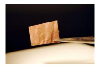
Copper structure shown here is a precursor material for explosive compounds used in military detonators. The copper structure can be formed on chips, then converted to an explosive compound. The compound is being used to improve US Navy detonator devices. Credit: Gary Meek
