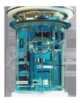
The sinker lies on a holder whose weight is compensated by the buoyancy of a hollow sphere and of an adjusting weight. Credit: PTB
