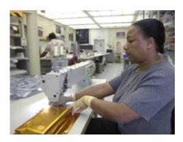
After cutting the raw material needed for the thermal blanket, technician Brenda Estavia carefully sews on a piece of Velcro. Click image for enlargement. Credit: NASA
