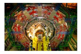
Installation of the world's largest silicon tracking detector in the CMS experiment at CERN.
