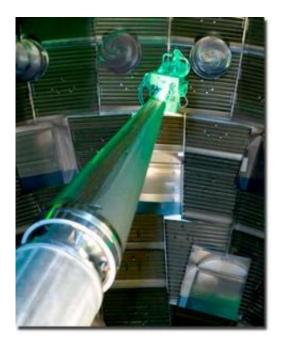
The Final Optics Damage Inspection system is mounted on a retractible arm inside the 30-meter diameter NIF target chamber.
