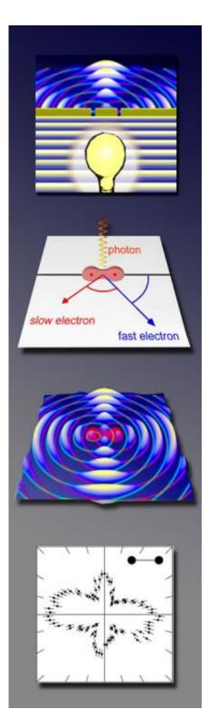
The traditional double slit experiment uses a single light source and two slits in an opaque screen (top). Compare to a double slit experiment using double photoionization of the hydrogen molecule (lower panels): when an x-ray photon ejects both the molecule's electrons, the two proton nuclei act as slits, causing
