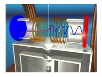
To perform the experiment, a supersonic jet of hydrogen (source at bottom) is ionized by a beam of x-rays from the Advanced Light Source (not shown). The doubly photoionized molecule blows apart, and the protons (red) strike the detector at left while the electrons (blue), trapped in a magnetic field, strike the detector at right. The energy of all the particles and the original orientation of the molecule can be determined from the measured results.
