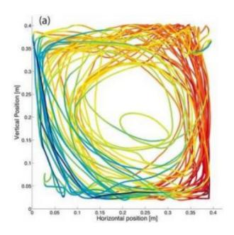
The path of a smart particle is color-coded to indicate the temperatures it wirelessly reports back during its travels. Credit: Y. Gasteuil, W.L. Shew, M. Gibert, F. Chill'a, B. Castaing and J.-F. Pinton
