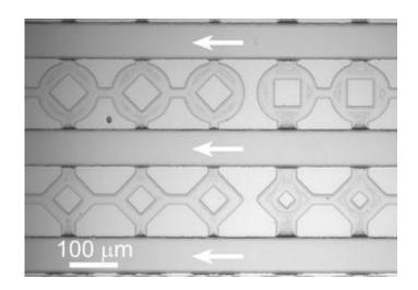
Image of microchamber device. Arrows designate the direction of flow in the microchannels. Image Credit: Kyle Campbell, UCSD
