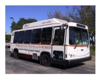
The 22-foot bus runs on batteries and a hydrogen fuel cell and emits just water vapor out of its tail pipe. The Center for Electromechanics at The University of Texas at Austin and the Gas Technology Institute will test this bus and other vehicles and technologies that reduce emissions and use alternate forms of energy.
