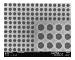
Scanning electron micrograph of tantalum pentoxide photonic feedback structures
