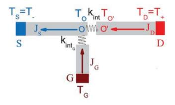
A thermal transistor controls heat flow. Heat passes between terminals S and D for the "on" state, and little or no heat passes between S and D for the "off" state. G is the control terminal. Image credit: Wang and Li.
