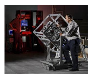
Nick Mascarenhas, physicist and principal investigator, prepares the detector for a test. The neutron scatter camera detects radiation at significant standoff distances and through shielding, and pinpoints radiation sources. (Photo by Randy Wong)
