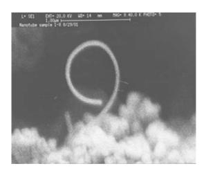
NASA Goddard's manufacturing process for single-walled carbon nanotubes, such as this one, is less expensive, simpler and safer than other methods. Credit: Innovative Partnerships Program Office, NASA GSFC
