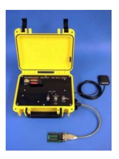
The data logger pictured can take 10,000 samples per second, provide researchers with a precise GPS timestamp for every measurement taken, and it records information directly to a USB jump drive. The data logger was designed and built by staff at the Geophysical Institute Electronics Shop. The Geophysical Institute is located at the University of Alaska Fairbanks. Credit: Geophysical Institute Electronics Shop photo
