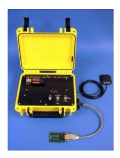
The data logger pictured can take 10,000 samples per second, provide researchers with a precise GPS timestamp for every measurement taken, and it records information directly to a USB jump drive. The data logger was designed and built by staff at the Geophysical Institute Electronics Shop. The Geophysical Institute is located at the University of Alaska Fairbanks. Credit: Geophysical Institute Electronics Shop photo
