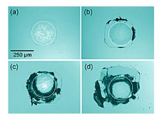
Optical micrographs of contact damage in silicon from cyclic stress show progressive damage after (a) 1,000 cycles, (b) 5,000 cycles, (c) 20,000 cycles and (d) 85,000 cycles. Color added for clarity, white circle shows computed size of the contact circle. Credit: NIST
