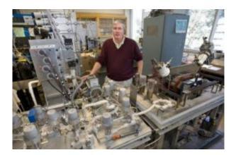
Berkeley Lab geochemist B. Mack Kennedy used this mass spectrometer (foreground) to determine helium isotope ratios in samples of surface fluids from the northern Basin and Range. Credit: Roy Kaltschmidt
