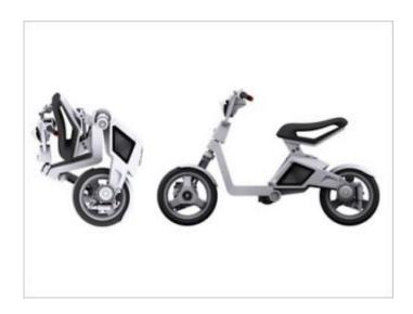
The MIT-designed electric scooter, shown folded up at left. Image courtesy / MIT Smart Cities Group
