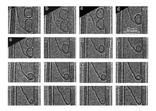
Atomic images of the inside of a nanotube show the formation of fullerenes, their reduction to C-60 buckyballs, and their dispersion when heated beyond that point. The images were taken by a transmission electron microscope. Credit: SNL
