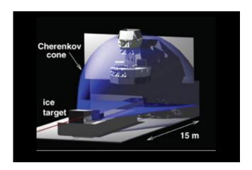
The ANITA probe visited SLAC in June 2006 for calibration tests using the accelerator beam and a block of ice.
