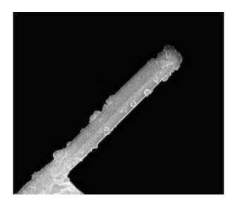
A one cubic micron sample of a microporous aluminium carboxylate. Credit: T. Loiseau, CNRS 2007
