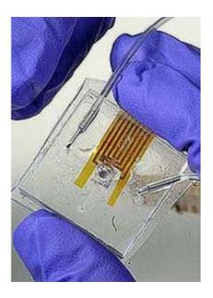
Johns Hopkins researchers have developed this thumb-sized microincubator. A syringe is used to inject living cells and nutrients into the device. Credit: Will Kirk/JHU
