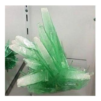
Ammonium dihyrogen phosphate, or ADP, crystals, which have applications in computer memory, laser and fiber optic technology. Credit: Florida State University
