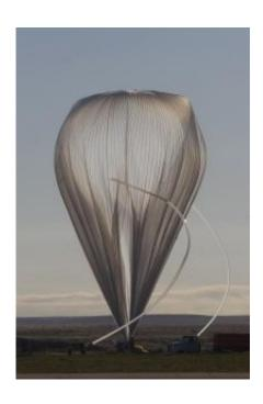
Slender hoses, blown into arcs by the wind, partially fill the balloon with helium before launch. A large portion of the balloon is left unfilled so it can expand as it ascends into the stratosphere, where air pressure is considerably lower. Credit: Carlye Calvin
